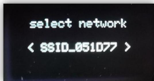
Using the rotary-click knob, you can enter the password in the next step. By long-pressing the button, you reach the sub-items "Back" and "Done". Ensure that a connection to the home network is possible and a good signal reaches the FG module.
