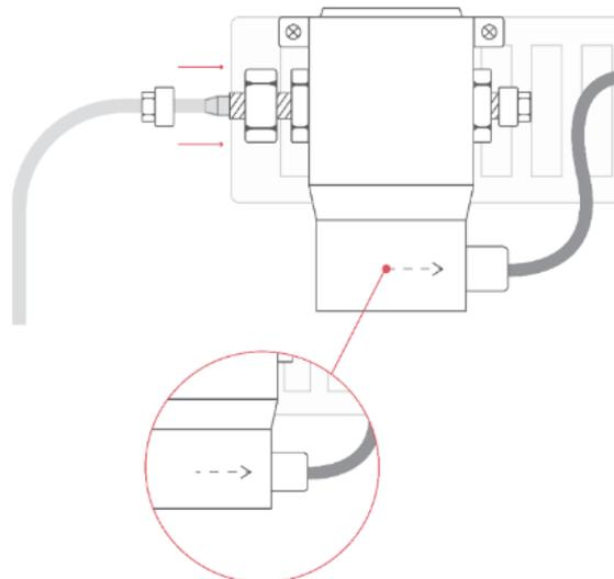
**ATTENTION:** Newer versions also have a black stopper on the CO2 valve. The hose must be connected to the connector on the opposite side of the stopper and tightened with the screw. The stopper can be left as it is. CO2 will still flow out.
