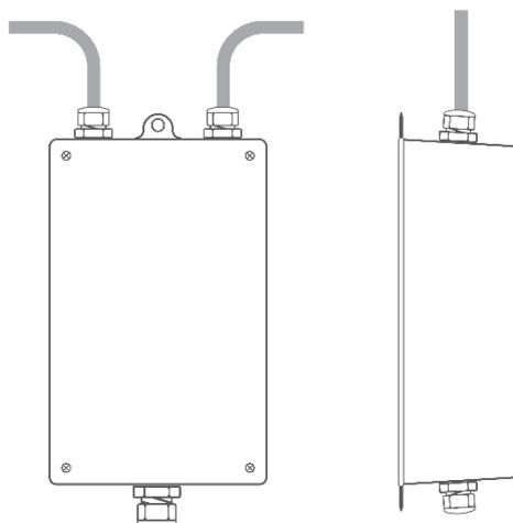
Then take the cable that you previously pulled through the drain hole and should be lying behind the box. This cable has 4 wires in different colors. The cable with the wires is then inserted through the cable gland (large gray screw in the middle, opposite the other two gray screws). The cable gland must be opened and later closed again. It can be opened and closed by turning.
