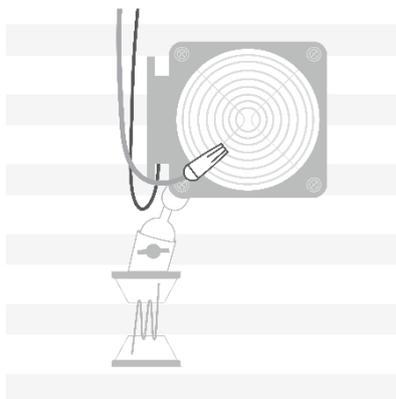
Tip: Use the supplied cable management to organize and neatly mount the fan, sensor, and module cables.
