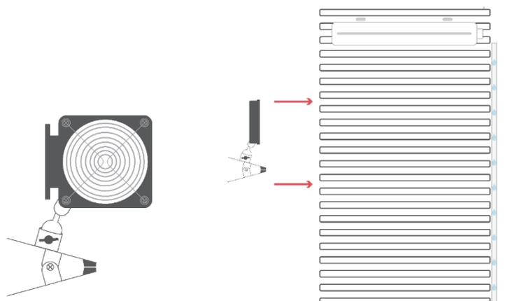
The direction of the fan can be changed using the adjustment screw. Adjust the fan so that it blows directly or indirectly onto the plants. This serves to strengthen the plants and remove the microclimate around the plants.
