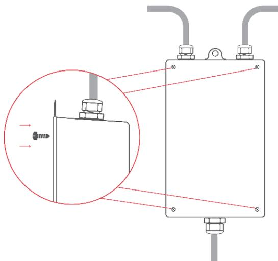
Once you have clamped all cables and secured the box against re-opening, you can plug the cabinet's power cable into the socket of the black terminal box. When this is done, plug the main plug into the power supply. The lamp may briefly light up.
