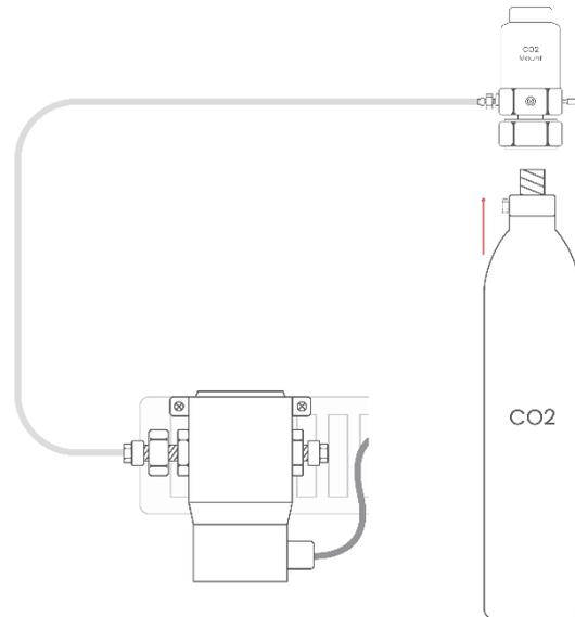
Then take the supplied wrench and place it on the bottom screw. Turn the CO2 bottle in with a jerky motion and some force. The wrench serves as a fixation here and can also be turned slightly in the opposite direction.
