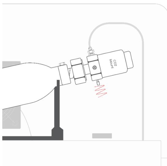
Place the CO<sub>2</sub> bottle on the supplied bottle holder. The CO<sub>2</sub> system is now complete and ready for use. Ensure that the bottle and bottle holder are securely placed and protected from tipping over.
