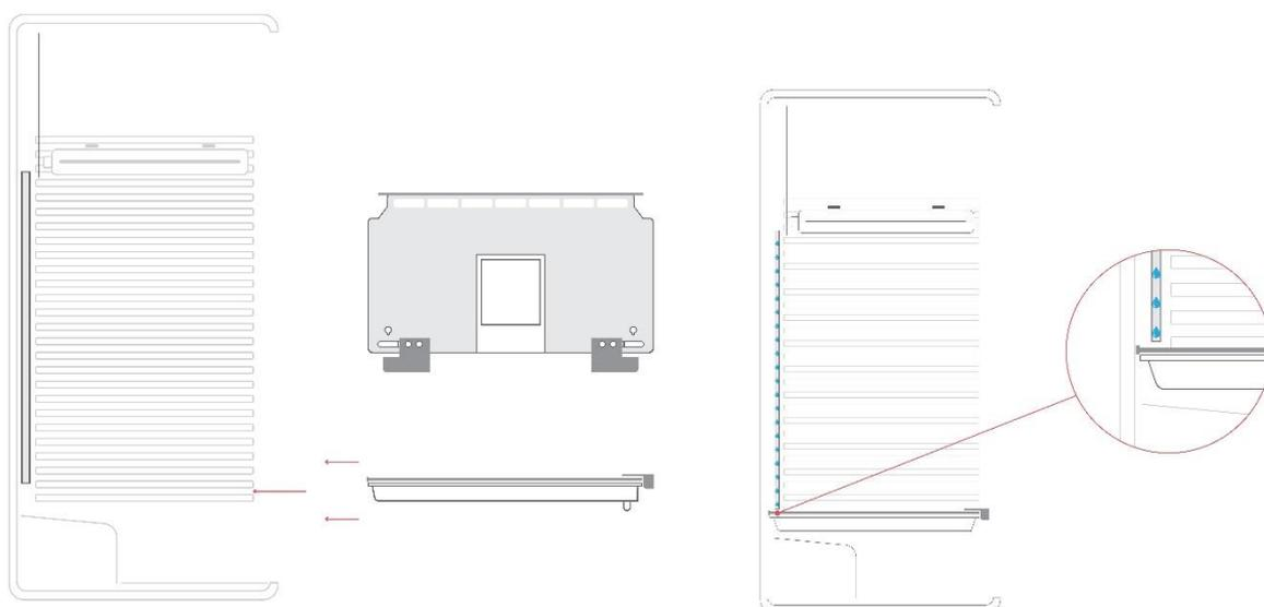
Then slide the two sliders into the side recesses in the door so that the condensate tray is fixed there and the seal on the back is firmly pressed against it.
