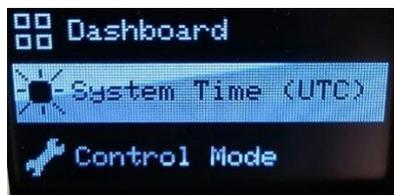
**Attention:** If the module has a connection to the internet, this time does not need to be set separately. In this case, the module automatically gets the correct time.
