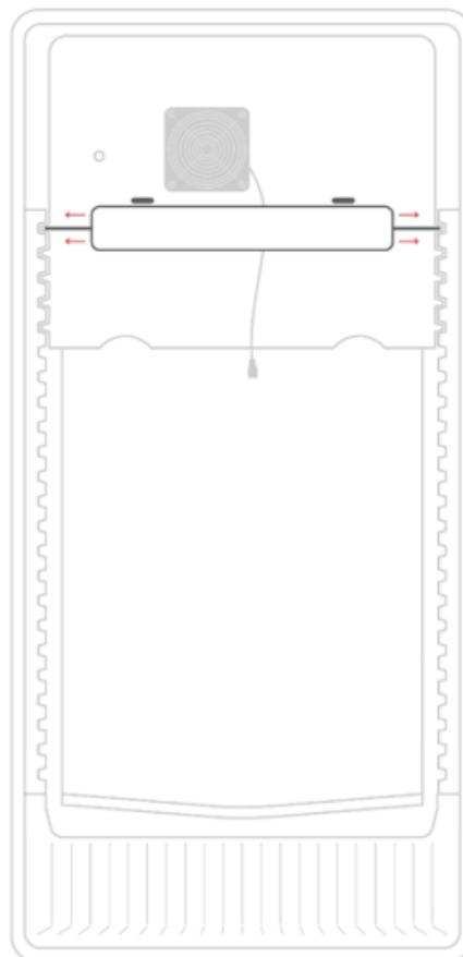
The rods must fully touch the interior walls to prevent slipping. When the module is securely held, tighten the screws on the top again.
