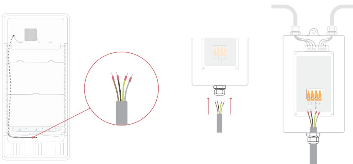
Once the cable has been inserted, you will see a terminal strip with labeled inputs. Insert the colors into the designated holes of the terminal according to the labeling.
