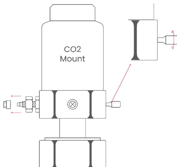
Plug the CO2 hose onto the connector, slide the screw onto the thread, and tighten it firmly. Ideally, the screw is tightened with a wrench or pliers, but usually tightening it by hand is sufficient.
