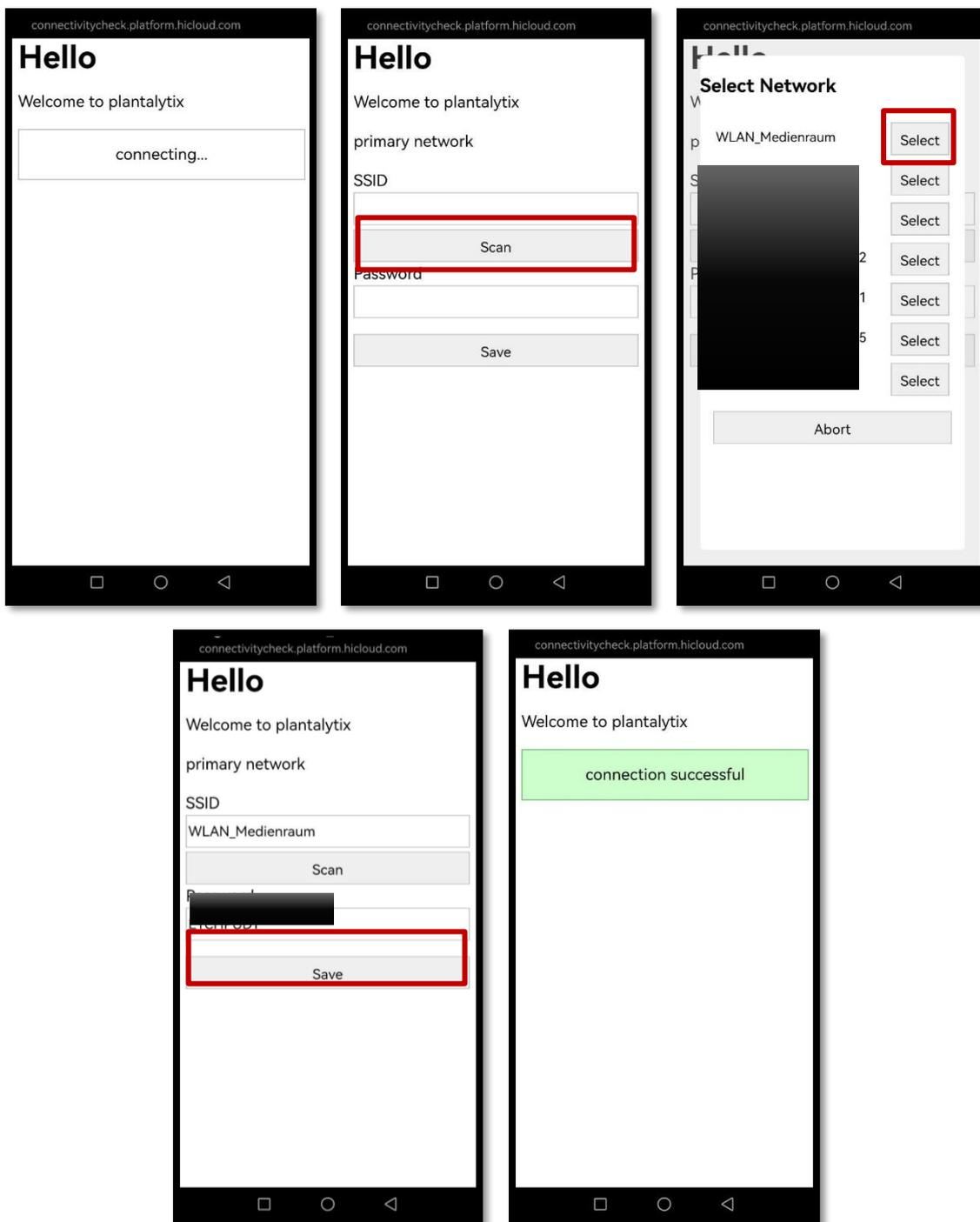
The FG module then attempts to connect to the home network and thus to the internet. If the connection is successful, a green box with "connection successful" will be displayed. If this is not the case, check the SSID and password again and enter them again. If this step was successful, the FG module is connected to the home network or the internet, and the portal can be used.
