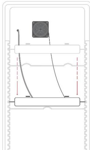
Then slide the module back into the top groove to simplify the subsequent steps. Now insert the other two rear wall parts so that the cutouts fit into each other. Push them all the way back again. The rear wall parts should ultimately merge seamlessly. Next, push the cable through the drain hole and push it downwards. The cable can then be pulled out at the back of the cabinet (at the very bottom).
