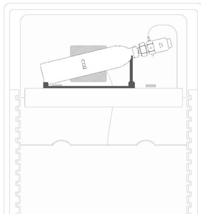
Next, the screw (fine needle valve) on the pressure reducer must be opened again so that CO<sub>2</sub> can flow from the bottle. Since the CO<sub>2</sub> valve is closed without power, you should not hear any hissing. Check all screws and connections of the CO<sub>2</sub> system again and then open the screw on the pressure reducer by 3 turns (3 complete rotations).
