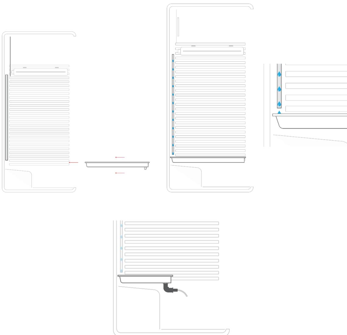
So that the condensate tray can be pushed all the way to the back, the cable that you should have in the bottom left corner must be placed in the cutout of the condensate tray.
