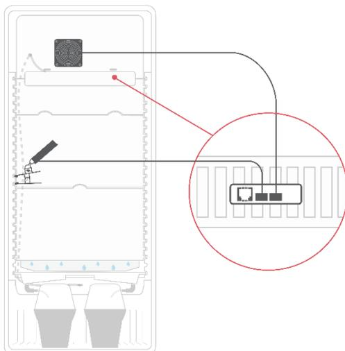
In the next step, the sensor cable (white cable coming from the back of the insert with a plastic cover mounted at the end) can be mounted into the bracket on the fan.
