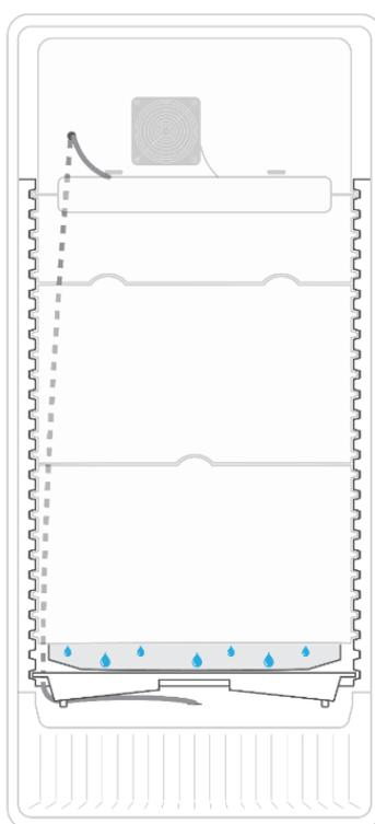
Regularly check during later operation whether there is any water below the condensate tray. If this is the case, it may mean that the condensation is not running back into the tray.
